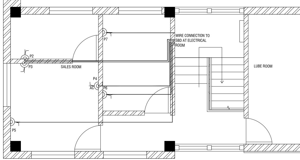
First Floor power point with conduit layout
