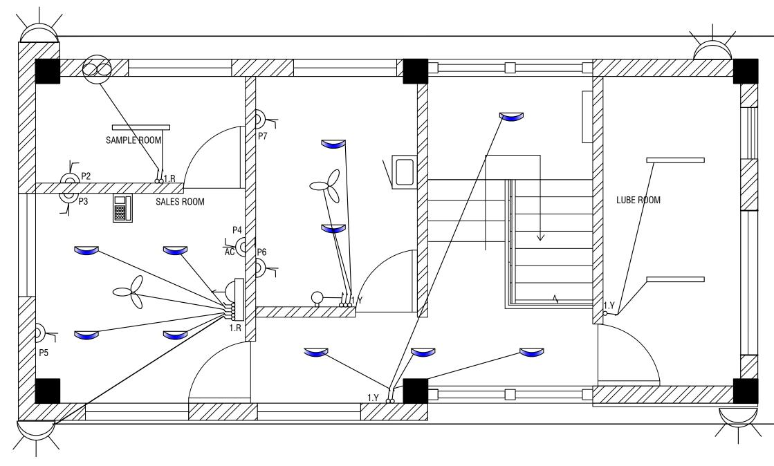
First Floor Fitting and fixture with wiring layout
