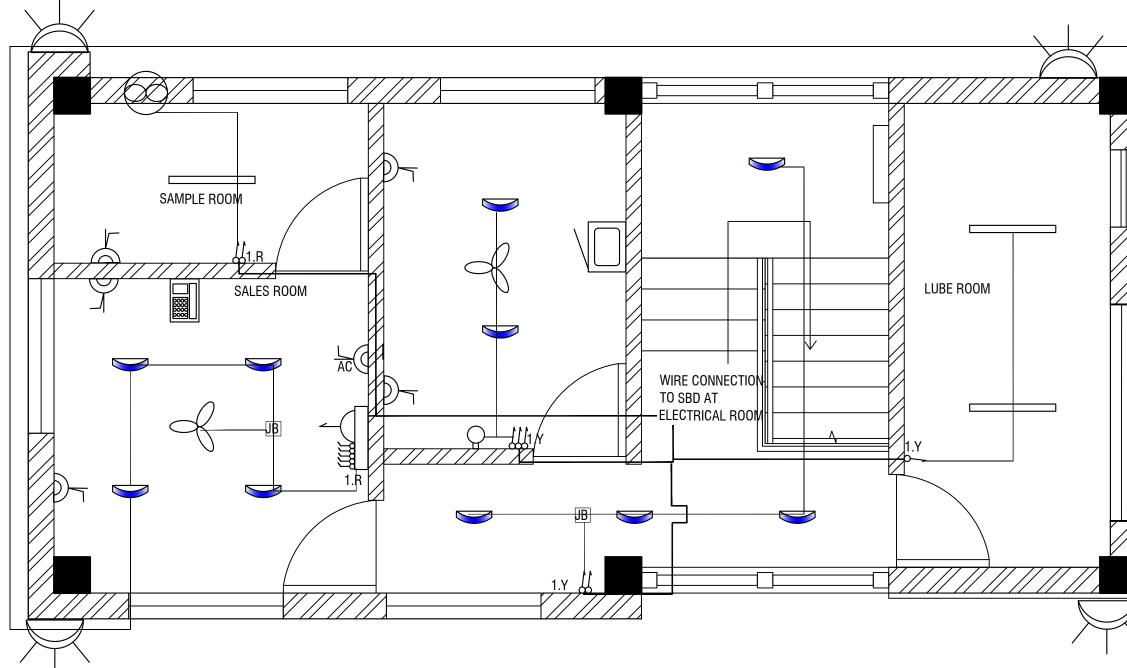
First Floor Fitting and fixture with conduit layo
