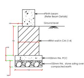
FOUNDATION SECTION DETAIL **BELOW PLINTH BEAM** (INTERNAL WALL)
