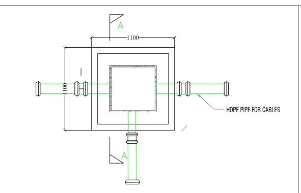
TYPICAL CONN. DETAIL (FOR 600x600mm CABLE CHAMBE
