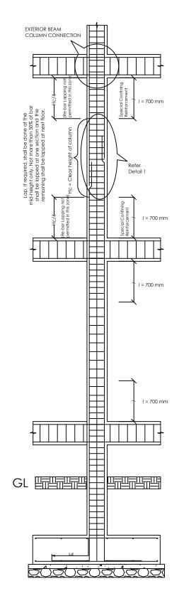
TYPICAL SECTION INTERIOR (showing typical arrangement of rebar and ties in columns)
